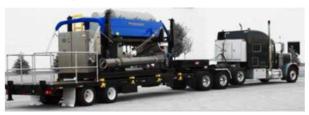
Many municipal and industrial wastewater treatment facilities need just one mobile Centrisys dewatering system: they simply move it between plants as needed for sludge dewatering and thickening. Only power and process connections are needed for system start-up and mobile centrifuge dewatering capacities ranging from 5 to 700 gpm (1 to 90 m³/h). The entire range of Centrisys decanter centrifuges is available for trailer-mounted mobile systems.
