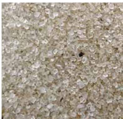
Struvite crystals are removed from the digested sludge and used as a beneficial fertilizer
